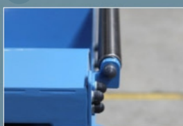
4 Optional installation of the second transport roller
